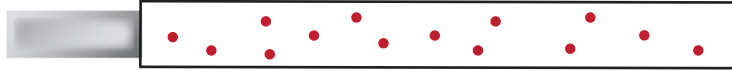
Fig. 4. A sketch of the “quasi-1D” model. The left part in grey represents an infinite-length ideal lead supporting M propagating modes. The disordered part is of a finite length L and contains finite concentration of random impurities inside.
