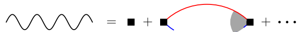
FIG. 3. Equation for the disorder averaged fluctuation propagator. Solid (red) line is the retarded and dashed (blue) line is the advanced Green's function. The black dot denotes the electron-electron interaction vertex, and the gray sector stands for the disorder-dressed vertex shown in Fig. 4.
